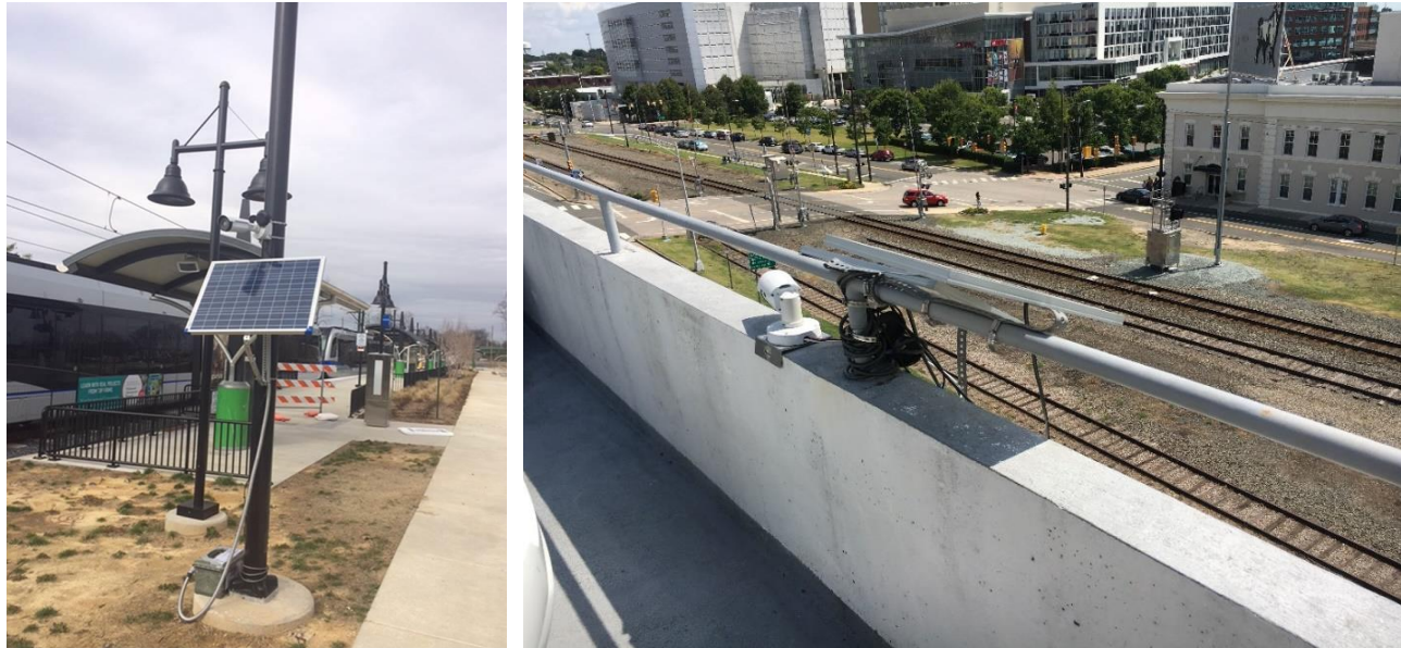
EXHIBIT 1. TYPICAL STATIC THERMAL DETECTION SYSTEM SETUP
